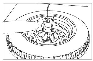
Tilt the retainer downward and through the center wheel opening. Make sure the retainer is fully seated across the underside of the wheel.
